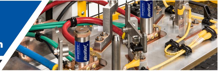
The VeriFast™ IA (Integrated Amplifier) Nut Detection Solution is CenterLine's latest system for monitoring weld pin position, an important part of the projection welding process.
